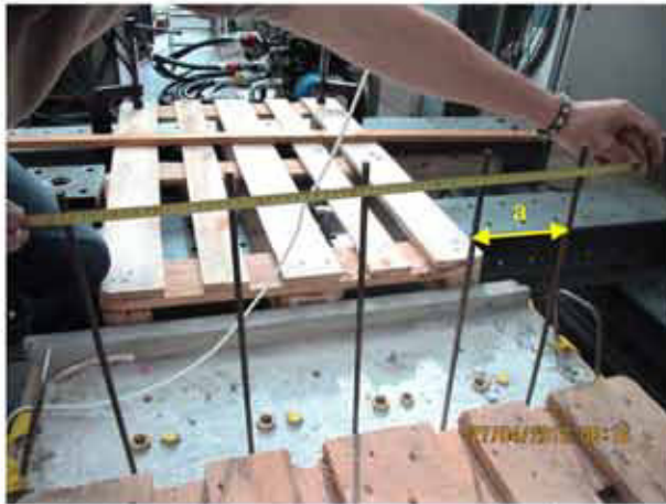
a) Arrangement of reinforcing bars, \varnothing 8 mm n=5 , a=150 mm, L=450 mm
