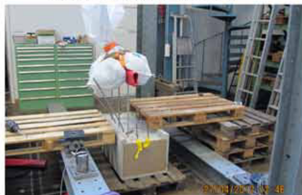
d) Test V03-14 (bar \varnothing 14 mm and bar spacing 300 mm)
