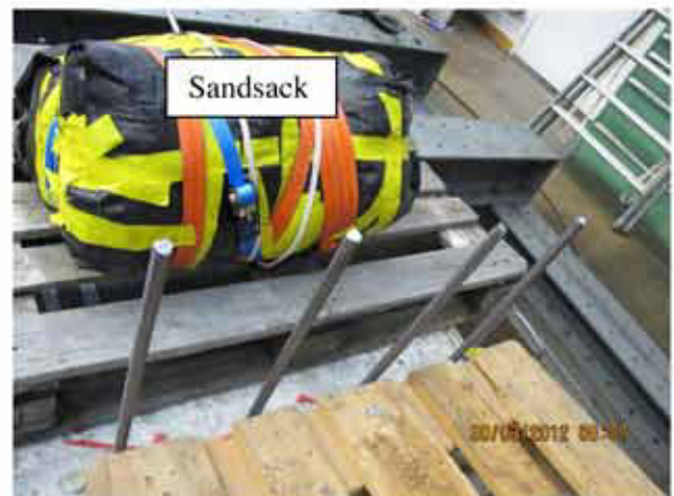
[Legend: Sandsack: Sandbag/ f) Arrangement of reinforcing bars, \varnothing 16 mm n=4 , a=200 mm, L=520 mm
