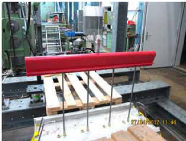
c) Arrangement of reinforcing bars, \varnothing 12 mm n=4 , a=200 mm, L=670 mm
