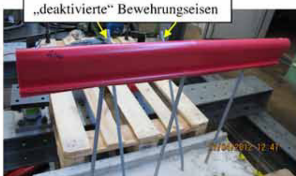
c) Test V03-12 (bar \varnothing 12 mm)
