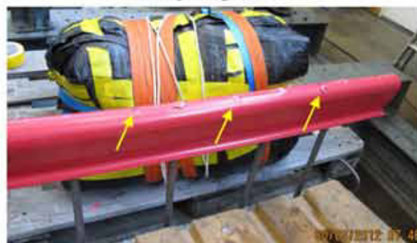
f) Tests V06-16 and V07-16 (bar \varnothing 16 mm) with the same strip Arrows show pressure points caused by test V06-16
