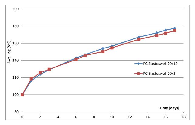
After 17 days the graph indicates that the swelling of PC Elastoswell 20x10mm and 20x5mm hasn't reached a maximum and constant value. The swelling will be observed the next days, untill the maximum is reached.
