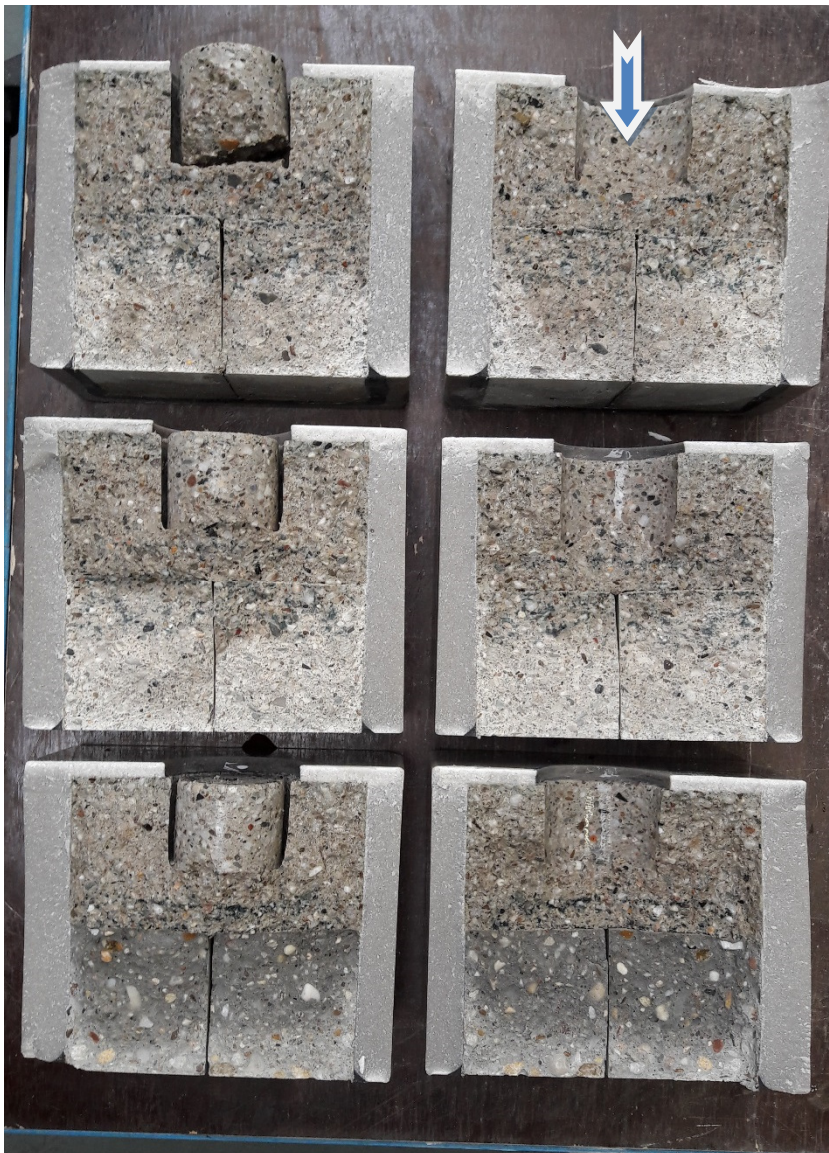
Photo 1. Sample 5 to 7, configuration B Fully saturated top and leakage with water at 7 bar after 24 hours
