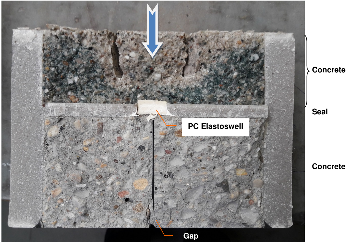
Photo 2. Configuration C, test piece is split after test. No leakage visible
